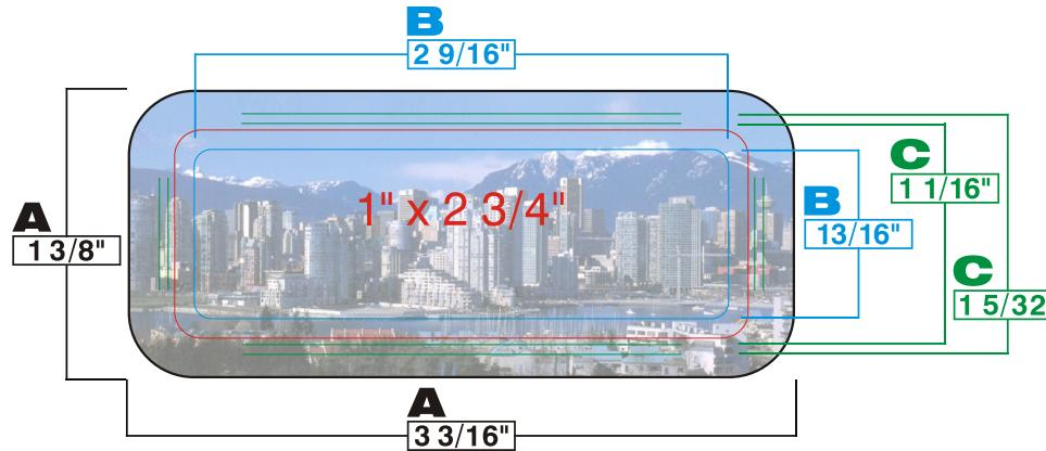
**A** - Cut line : must be in the button design.
