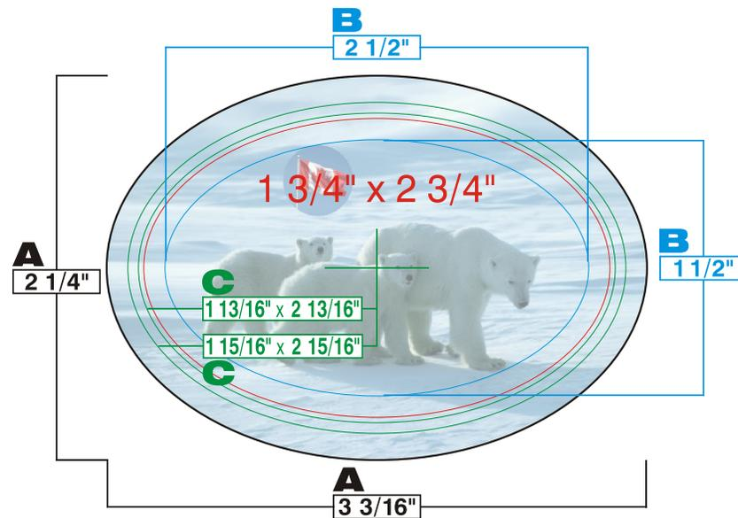
**A** - Cut line : **must be in the button design.** Background button design has to bleed to this line.
